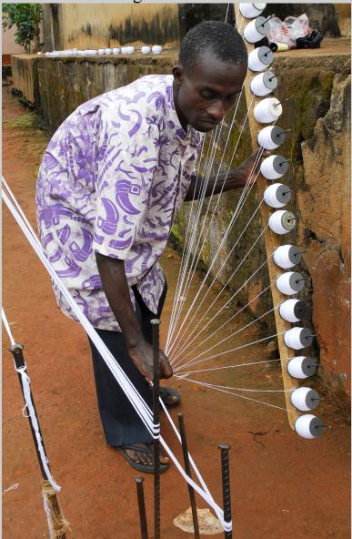
Figure 7.72c Steven Akwah (Ashanti) holds a creel in his left hand while crossing the threads around the end of a metal stake with his right hand to measure a kente warp in Adawomase, Ghana (photograph by Carol Ventura, 2009).
