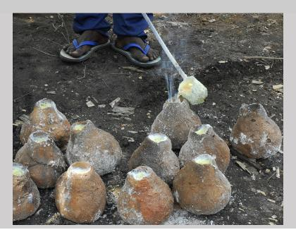
Figure 7.66f Brass is poured into molds in Krofofrom, Ghana (photograph by Carol Ventura, 2008).
