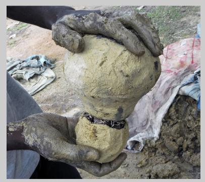
Figure 7.66d Adding a crucible of metal to the mold in Krofofrom, Ghana (photograph by Carol Ventura, 2008).
