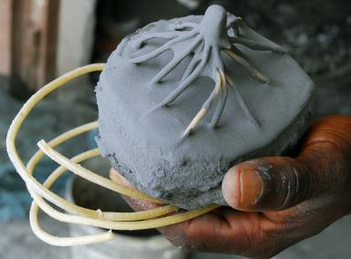
Figure 7.66c Wax covered with slurry in Krofofrom, Ghana (photographs by Carol Ventura, 2008).
