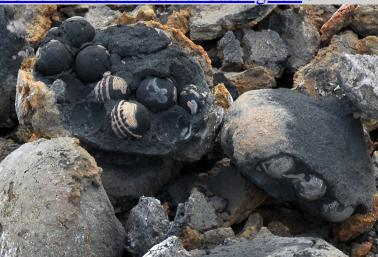
Figure 7.66g Warm molds broken apart to reveal the casts in Krofofrom, Ghana (photograph by Carol Ventura, 2008).
