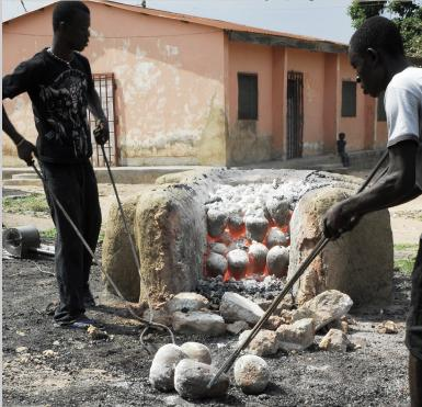
Figure 7.66e Removing hot molds from the kiln in Krofofrom, Ghana (photograph by Carol Ventura, 2008).
