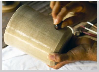
Figure 7.5a Patricia Martin burnishes an unfired earthenware pot with a quartz pebble to prepare it for painting. She then paints slip onto the surface to reproduce a pre-Hispanic vessel in Muna, Yucatan, Mexico (photograph by Carol Ventura, 2002).
