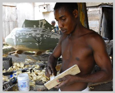
Figure 7.69e Aojer Dani Klur (Ga) applies glue before he nails the wood in place. A fish coffin in the background is almost finished at the Kane Kwei workshop in Teshie, Ghana (photograph by Carol Ventura, 2008).
