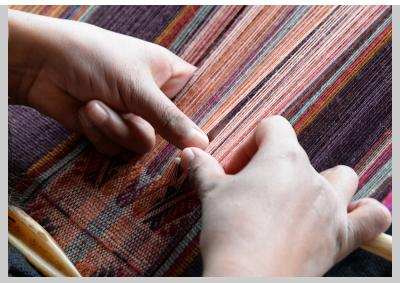
Figure 7.22g Picking up warp threads with a bone pick and fingers to create the shed. The warp is close together to create a warp-faced fabric that hides the weft in Pitumarka, Peru (photograph by Carol Ventura, 2017).
