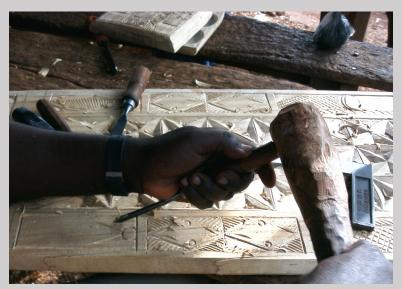
Figure 7.68a Carving a wood panel with mallet and chisels in Foumban, Cameroon (photograph by Andrzej Gutek, 2001).
