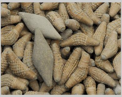
Figure 7.66b Wax covered cores in Krofofrom, Ghana (photograph by Carol Ventura, 2009).
