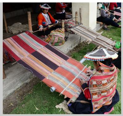
Figure 7.22f In the foreground, Ana Espinoza (Quechua) weaves on a backstrap loom set up with three discontinuous warps in Pitumarka, Peru (photograph by Carol Ventura, 2017).
