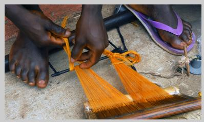
Figure 7.72f After threading the warp through the reed, Ofori A. Isaac (Asanti) ties bundles of warp around the metal rod that will be tied to the warp beam of the loom (under his feet) in Adawomase, Ghana (photograph by Carol Ventura, 2009).
