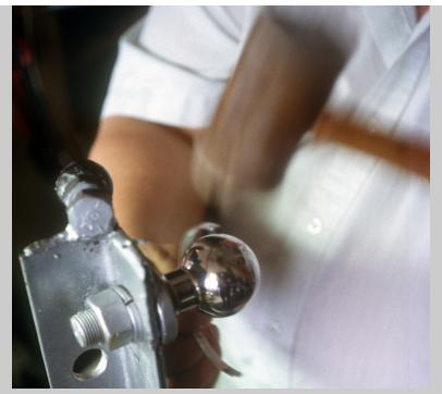
Figure 7.61c Dave Hunter (Haida) hammers the silver against a secured trailer hitch to shape it into a bracelet (photograph by Carol Ventura, 2001).
