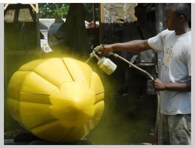
Figure 7.69g After all the joints between the pieces of wood have been filled, the coffin is sprayed with several colors of oil-based paint at the Kane Kwei workshop in Teshie, Ghana (photograph by Carol Ventura, 2008).
