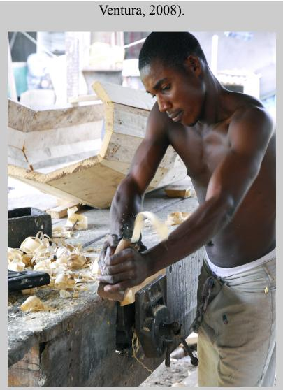
Figure 7.69c Aojer Dani Klur (Ga) planes each piece of wood to fit the coffin he is making at the Kane Kwei workshop in Teshie, Ghana (photograph by Carol Ventura, 2008).
